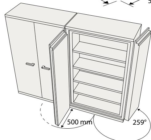
The cabinets of SA-series can be placed directly next to each other. Opening the doors 90 degrees will provide full access.
